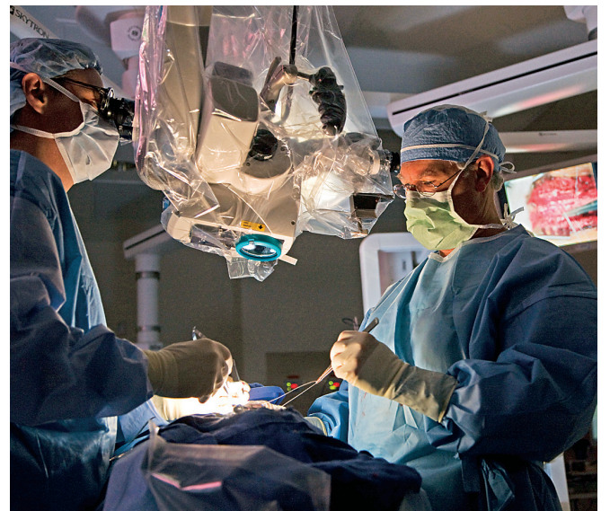
The Truevision 3-D surgical microscope converts optical view from the microscope to a digital 3DHD image, displaying video on monitors in the room.
